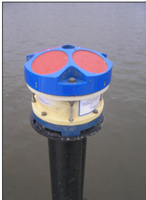
Fig. 3 Current meter ADCP WHM300-I-UG1
